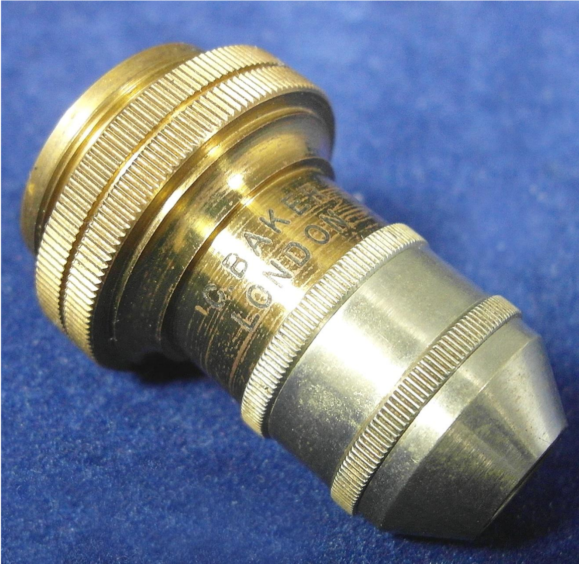
Figure 12. 1/2 Inch C. Baker Objective
